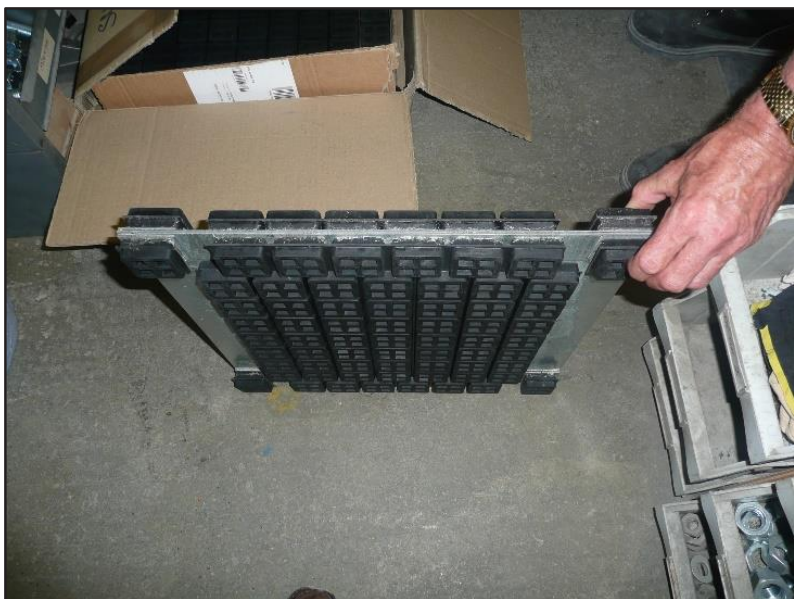
Noise-reducing pad inspection at factory
